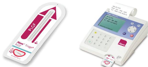
**Fig.2:** Placental growth factor (PIGF) measurement instrument.
